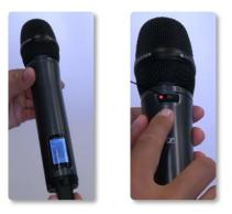
Turn on the microphone by pressing the **red button** at the bottom until the screen lights up
